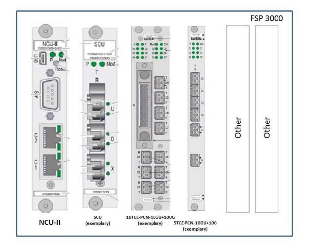
Figure 1.4 – NCU-II card in its operational environment
